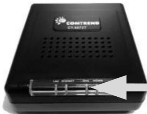
**A solid DSL light indicates a successful DSL connection**
